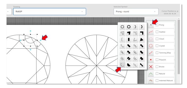
You can place each prong one at a time or expedite the process using the Arrange Prongs feature. Hovering over the prong symbol and right clicking will activate the Symbol menu. Choose 'Arrange Prongs'.
