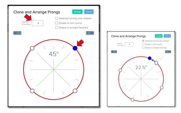
Click on the 'Arrange' button to complete prong propagation and return to the Plotting window.
